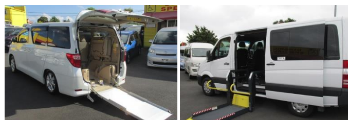
fig 3.5: rear transfer, side transfer
