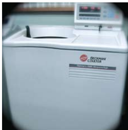
Beckman Coulter Ultracentrifuge for harvesting cultures at very high speeds (up to 100,000rpm). Purchased with New Zealand Lottery Grant.
