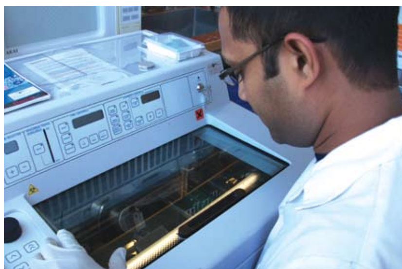
Microtome in a refrigerated chamber minus 20 degrees C- PhD student Praveen Parachuru freezing and cutting frozen tissue for Immunohistochemistry and Immunofluorescence
