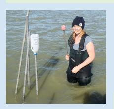
To measure this process, I have built flexible *in situ* chambers allowing tubidity from wave forces to be incorporated, and am tracing the transformation of nitrate to nitrogen gas using stable isotopes.
