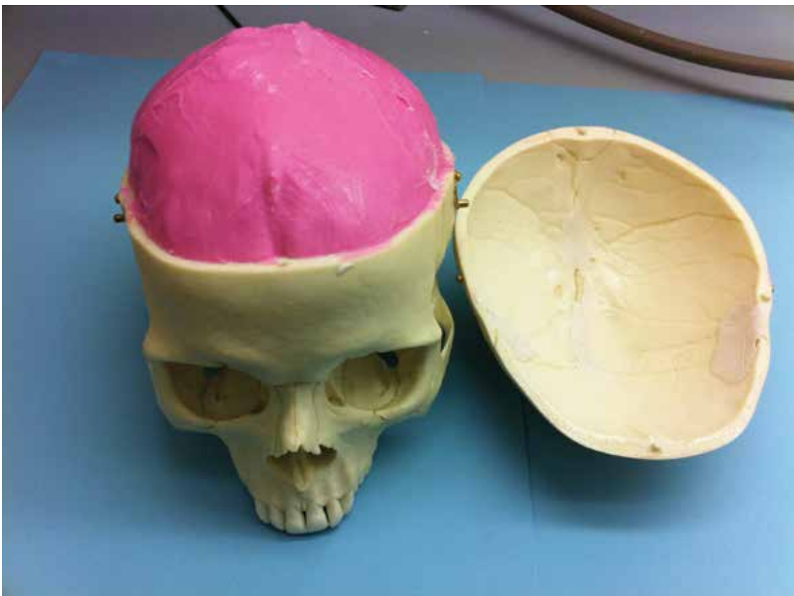
Moulding process of the brain cavity in the development of a simulant skin/skull/brain anatomical model for sub-concussive brain injury force transfer research.
