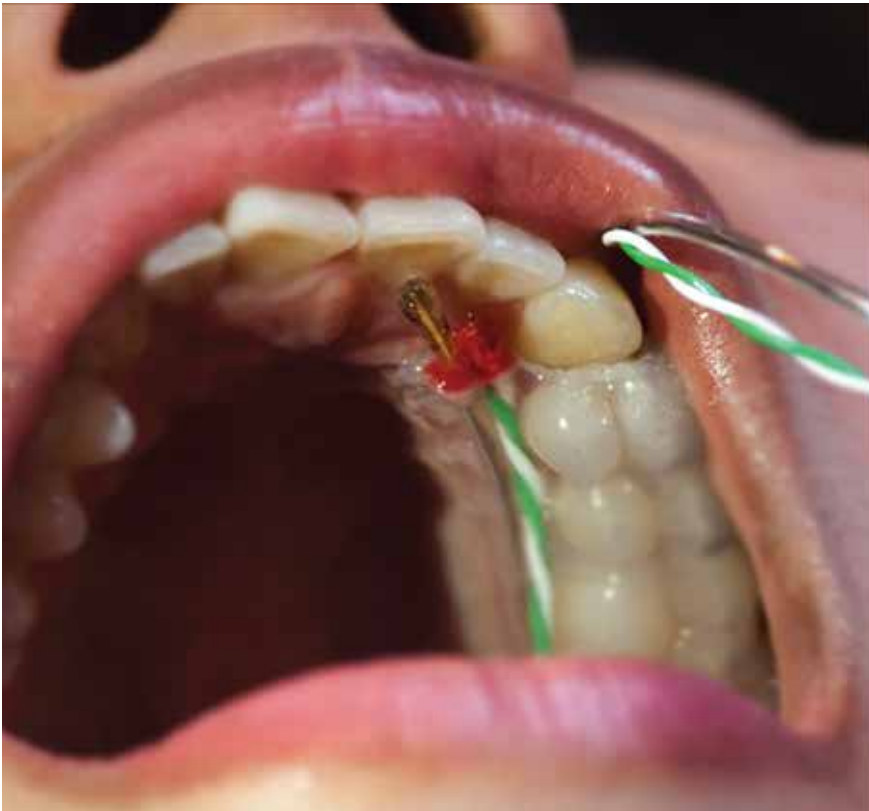
Developing intraoral sensors to monitor pH, temperature and jaw activity.
