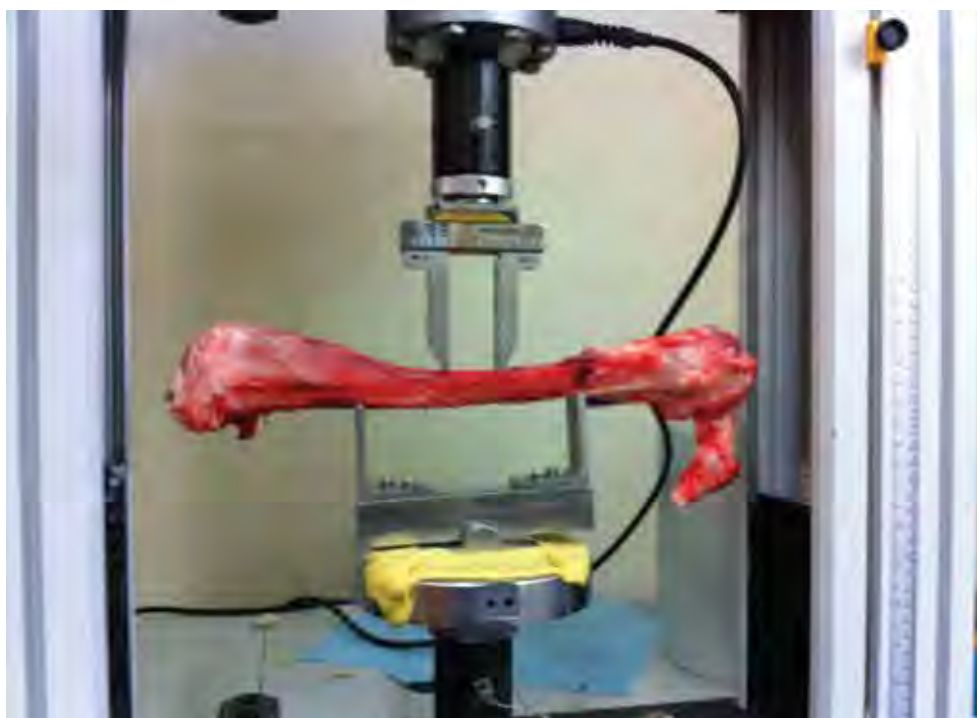
Image showing 4-point bending flexural strength testing of a fresh deer femur.
