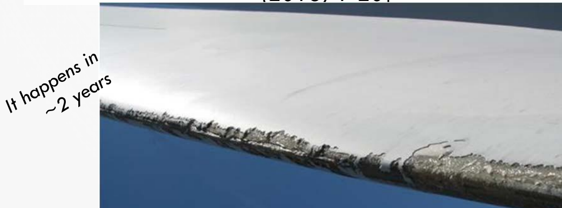
Leading edge erosion of a wind turbine blade
