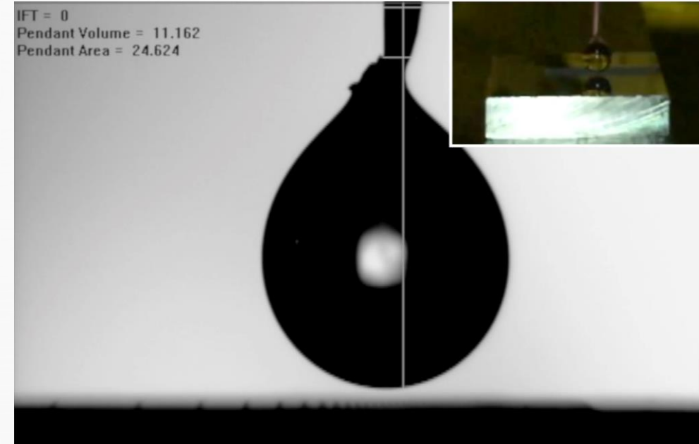
Spontaneous moving in Cassie-Baxter state (the droplet ends up in Wenzel state)
