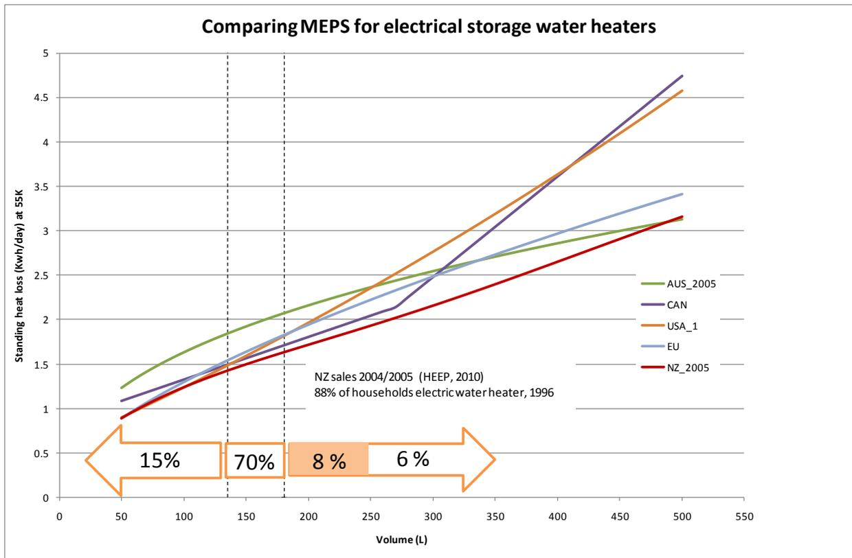
Figure 6. Maximum allowable heat loss rate (kWh/day at 55°C temperature difference) for electric storage water heaters plotted against volume (in litres) for 5 countries/economies (NZ, AUS, Canada, U.S, EU). Arrows indicate the market share of the different sizes of storage water heaters sold in New Zealand. Most prominent are those ranging between 135 and 180 litres (sale data NZ sales 2004/2005 from HEEP, 2010).
