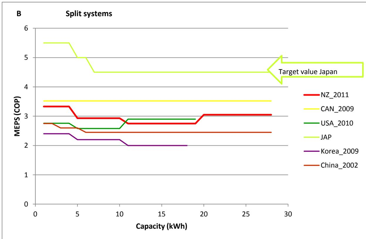
Figure 7: Minimum heating Coefficient of Performance depending on capacity (kWh) for single system heat pumps (A) and split systems heat pumps (B) for seven different countries (NZ/AUS, Canada, U.S, Japan, Korea and China).
