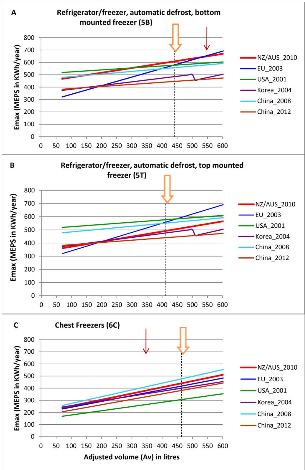
Figure 3. Maximum allowable energy consumption ( $E_{max}$  in kWh/year) for two different types of refrigerator-freezers (5B and 5T) and chest freezers (6C) for five countries (NZ/AUS, EU, US, Korea and China). Orange arrows indicate average size of the most often purchased models in New Zealand; red arrows indicate the same for Australia.
