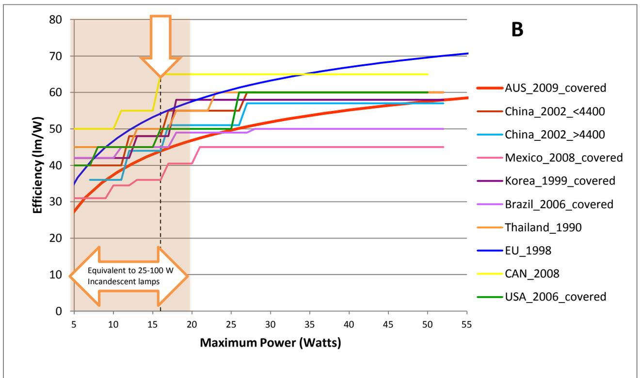
Figure 5. Minimum energy efficiency standards (in lm/W) for covered (A) and bare (B) compact fluorescent lamps for eight different countries (Australia, China, Mexico, Brazil, Thailand, EU, Canada and California). The arrows indicate the most purchased CFLs in Australia (16 W) and the most important product range (equivalent to 25-100W incandescent lamps).
