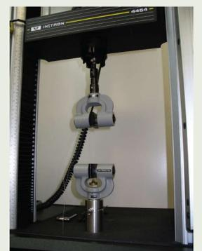
Fig. 6. Tensile testing to measure fibre aggregate strength (tenacity). Test length 100 mm.
