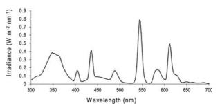
Fig. 1. Spectral output (300–700 nm) of all light tubes combined in the laboratory set-up (W  $\rm m^{-2}\,nm^{-1}$ ) as measured by the LiCor Li-1800UW spectroradiometer.
